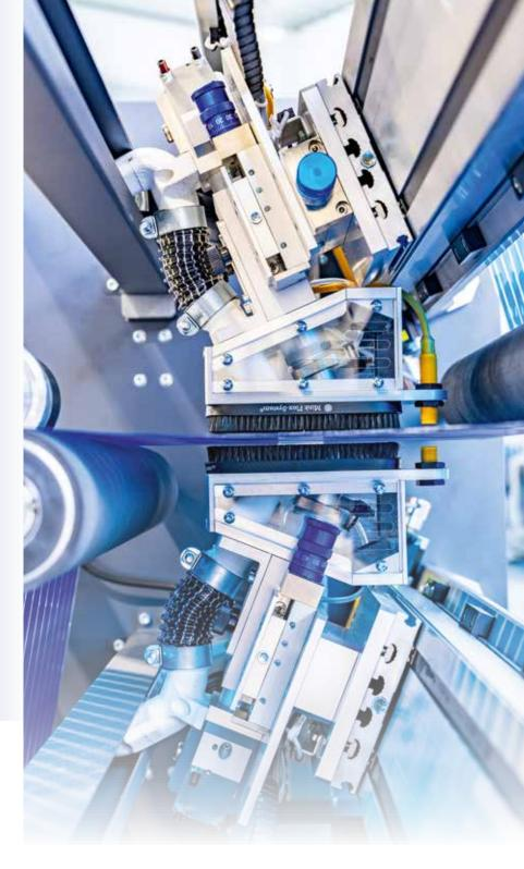
perforation ensures precise and consistent results, optimizing the packaging process for maximum product freshness and quality.
